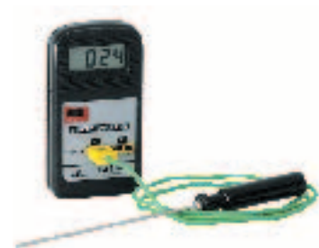
Temperature gauge for RAKU 100, easy to operate, NiCr-Ni temperature sensor, display range 20 – 1200 °C, optional connection of second sensor with display changeover
