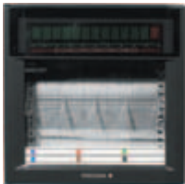
Data recording station with data diskette storage and graphic process display
