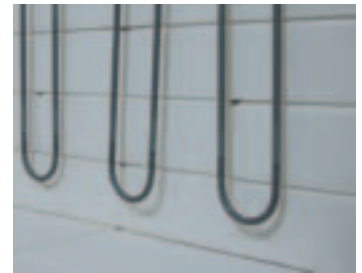
Furnace chamber lined with solid lightweight refractory brick insulation instead of fibre material for melting tests in the laboratory
