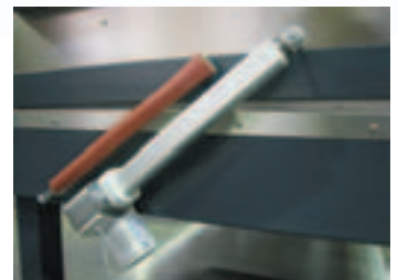
Automatic lid opening via electromechanical spindle
