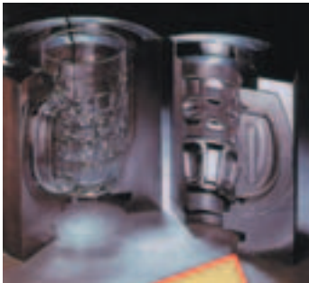
Mould for production of beer glasses
