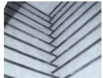
Heating from 4 sides with SiC rods
