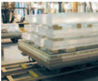
Shuttle kiln in customized dimensions for tempering quartz rods
