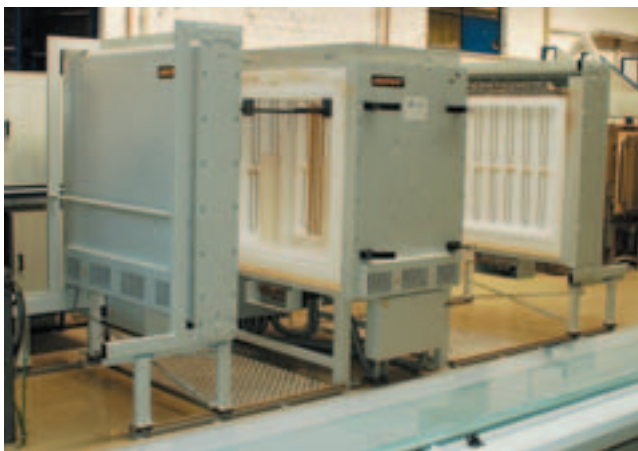
Dividable high-temperature furnace HT 1000/17S for sintering quartz glass tubes
