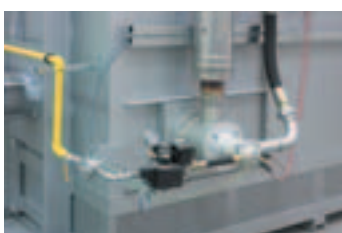
Indirect gas heating by radiation tubes
